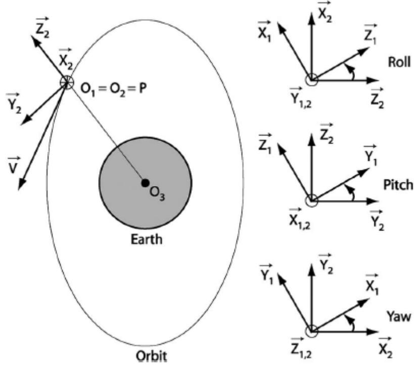
Figure A2.2: Orbital coordinate system and attitude variations.
