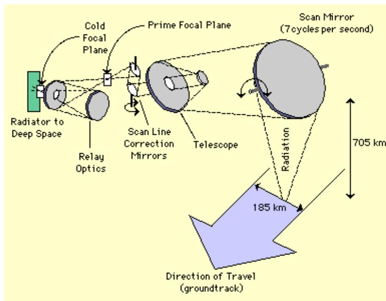
**FIGURE\_4. 8: Optical and meccanical subsystems in Landsat ETM+**
