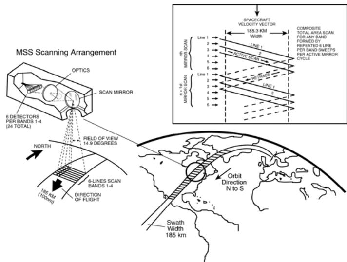
FIGURE\_4.4: MSS Scanning system [130]
