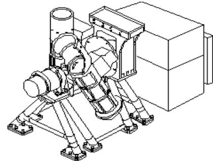
**FIGURE 4. 13: ASTER VNIR subsystem**
