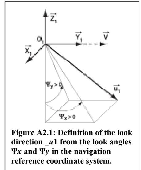
**Figure A2.1: Definition of the look direction  $\vec{u}_1$  from the look angles  $\Psi_x$  and  $\Psi_y$  in the navigation reference coordinate system.**
